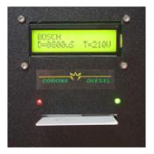
The simulator is able to direct 6 piezo electroinjectors by running a test bench simulation as it was in the engine; The CD555 Common-Rail Simulator would pilot the pump while performing delivery and pressure test (0-2000 Bar). Unlikely the others, this is a specially designed system for checking piezo stone consumption and carrying through a complete mechanic and hydraulic screen (not the 0-300 Bar injector test).
