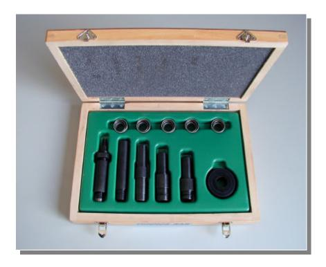
Tool box is equipped with 6 pieces for assembling and dismounting the radial-jet pump bearings and 5 bearing kit.
