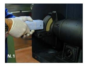
The cleaning and polishing brush (*P.n.SICR*) fits a grinding wheel. The center hole can be anlarged to fit your equipment.Before using the brush must be immersed in diesel fuel for one hour, followed by squezing excess fuel.
