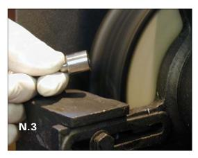
The brush is indispensable for polishing top surface of the nozzle and the injector body preventing leakage. This method of polishing also not not damage the surface, which happens with the old method of hand polishing (see photo 3-4)
