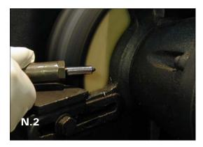
It is possible to clean and polish new nozzle types (also the Common-Rail) without damaging the nozzle holes.
