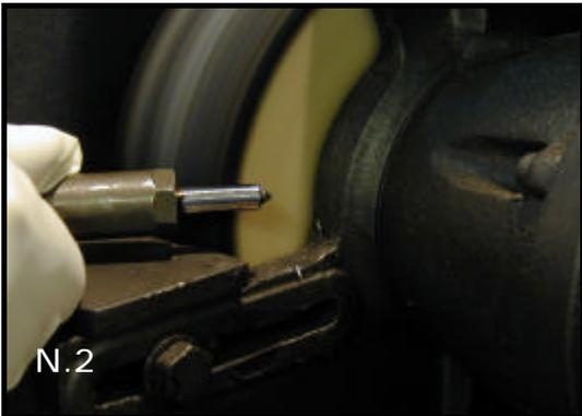
It is possible to clean and polish new nozzle types (also the Common-Rail) without damaging the nozzle holes.
