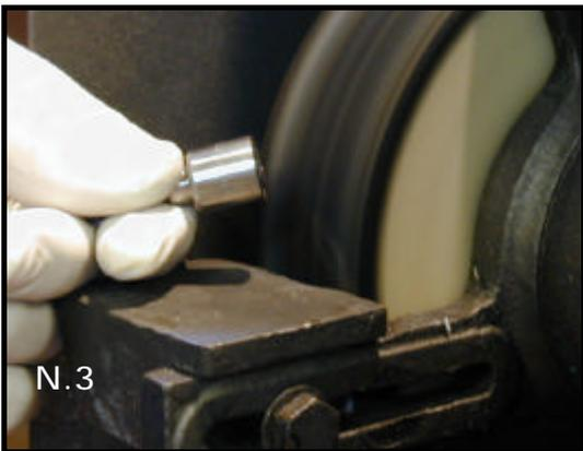
The brush is indispensable for polishing top surface of the nozzle and the injector body preventing leakage. This method of polishing also not not damage the surface, which happens with the old method of hand polishing (see photo 3-4)
