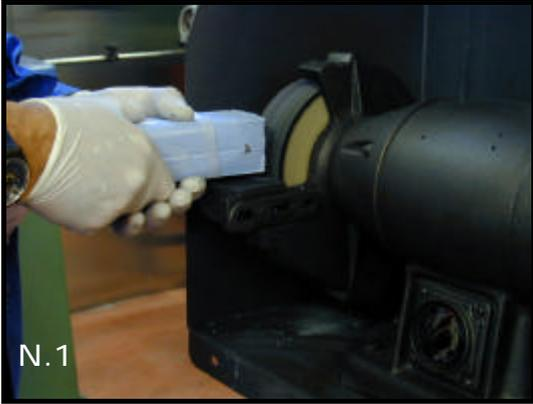
The cleaning and polishing brush (No.SICR) fits a grinding wheel. The center hole can be enlarged to fit your equipment. Before using the brush must be immersed in diesel fuel for one hour, followed by squeezing excess fuel.
