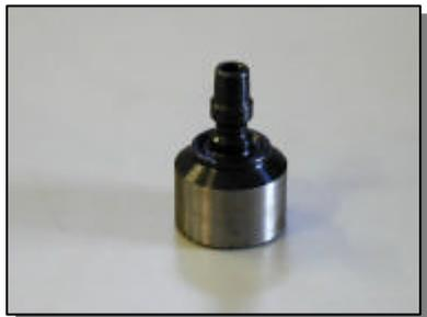
ADATTATORE BANCO DI PROVA HARTRIDGE NUOVO TIPO
