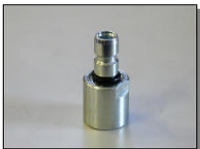
ADATTATORE BANCO DI PROVA BOSCH NUOVO TIPO
