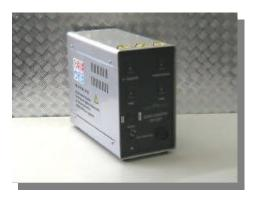
The tester has been designed to direct 6 electric-piezo electroinjectors and monitor on test bench where the engine is tested too.
