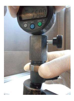
The tool must be connected to the *Q200-NS* solenoid depth measuring tool
