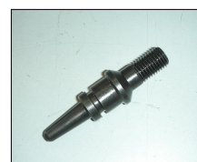
Needle for injector gauge block P.N.: 555-41/U
